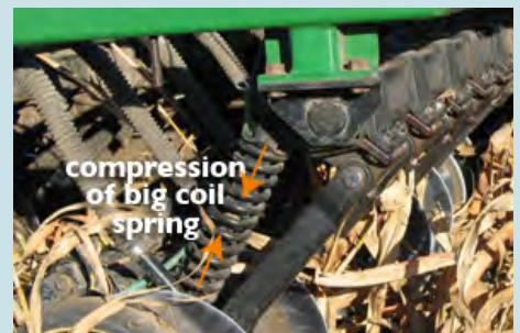
The only meaningful indicator of down-pressure being applied is inches of compression on this spring.
