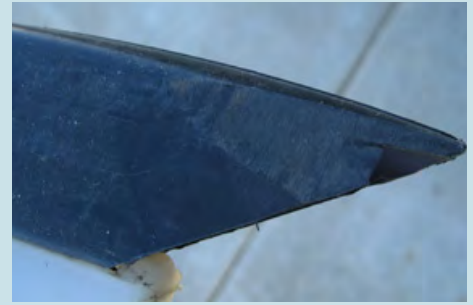
Frayed seed tube. The edges curl inward, and cause seeds to bounce erratically. Of course, this was due to a worn-out seed tube guard, which is itself causing even more problems with seed placement (furrow too narrow, sidewalls caving in prematurely as blades flex and unflex).
