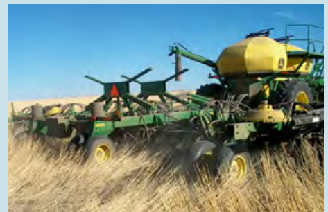
Weights located for maximum mechanical advantage on Deere 1890 drill, on 10-inch spacing. This is in Alberta. More southerly soils with poorer structure and lower OM (organic matter) will require more.
